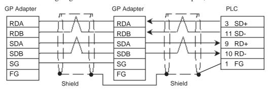
• When using Digital's Multi-link Cable, GP230-IS12-O
