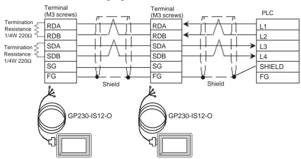
• When using Digital's Multi-link Cable, GP230-IS12-O
